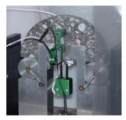
**Figure 6.7: The SCB test**
