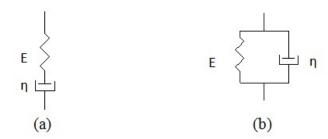
Figure 9.7: Maxwell Model (a) and Kelvin-Voigt Model (b)
