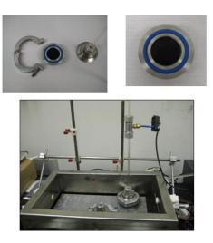
Figure 12.1: Dilatometric system used to measure glass transition temperature (Tg) of asphalt binders
