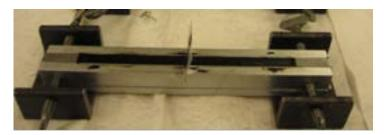
Figure 10.3: SENB specimen mold
