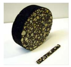
Figure 9.2: IDT and BBR test specimens
