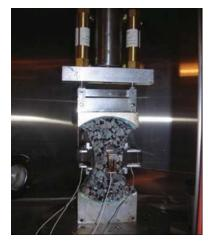
Figure 2.4: Dog-bone direct tension test prototype (27)
