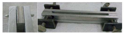
Figure 10.7: Modified SENB mold system with alignment pins
