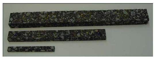
Figure 2.2: 1x, 2x, and 3x asphalt mixture beam specimens. (17)
